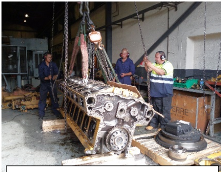
Turning the No. 2 engine block to remove pistons and liners
