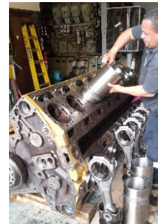
Installing cylinder liners
