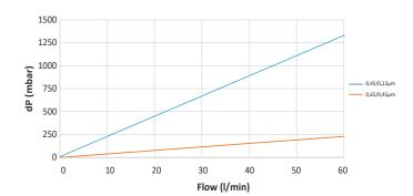
Note: 10" cartridge tested with water @20°C, 1.005 cP (typical flow rate)
