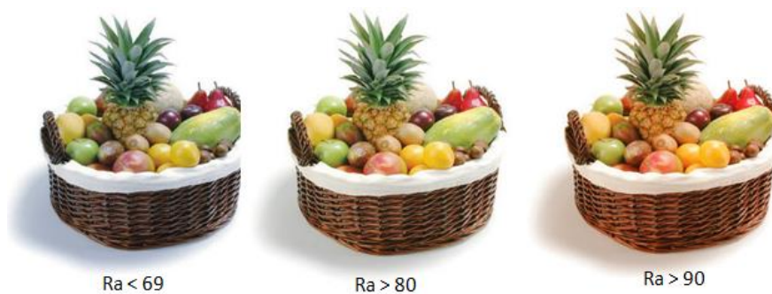
Figure 3: Example of color rendering by artificial light and how it is perceived by the human eye at different Ra values
