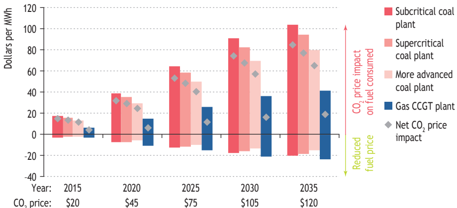
Figure 14.9 • Additional price impact of the cost increase to the electricity producer in selected OECD+ countries resulting from the CO 2 price in the 450 Scenario
