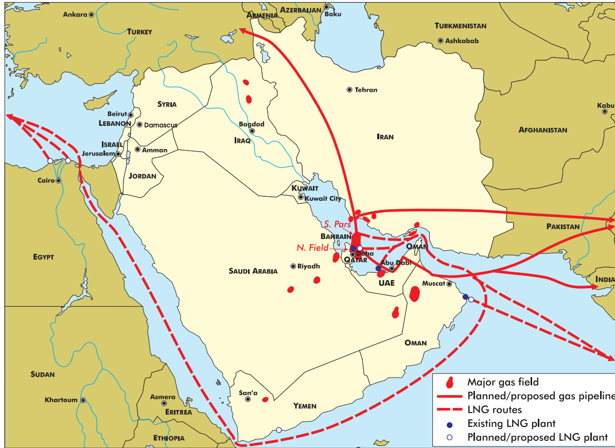
Figure 3.26: Inter-regional and Export Gas-Supply Projects in the Middle East
