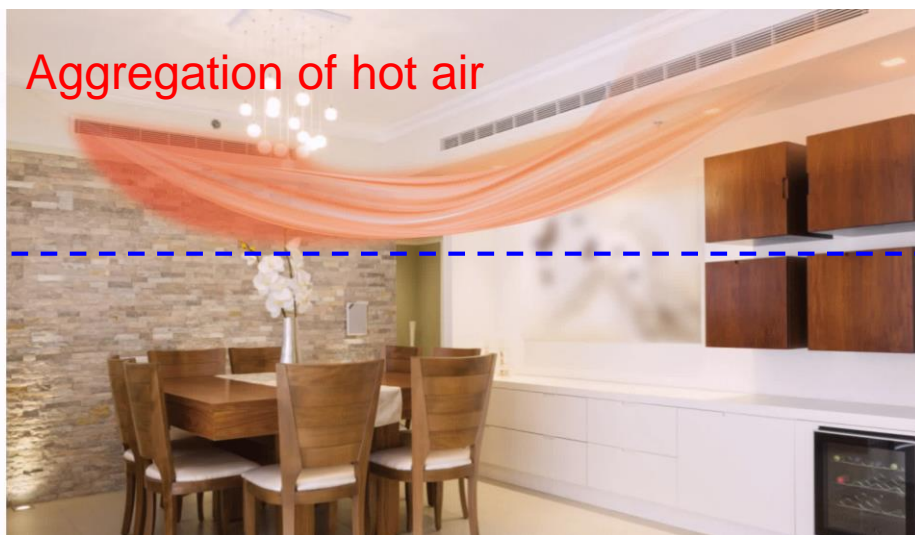
Uneven air distribution for the traditional air duct
