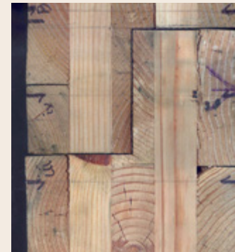
Mass timber performance problems are mostly moisture related. The SMART CLT project, led by Oregon State University (OSU) Assistant Professor Mariapaola Riggio and funded by the TallWood Design Institute (TDI), recently demonstrated that exposure to rain, followed by simulated interior conditions, can result in higher levels of checking and other stress-relief discontinuities, particularly at the edges where connections would occur.
