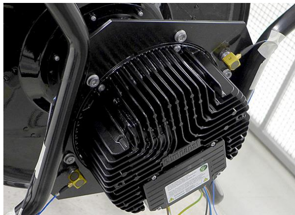
Figure 66: Triaxial vibration sensors (yellow) on fan (source: EBM-Papst, 2018)
