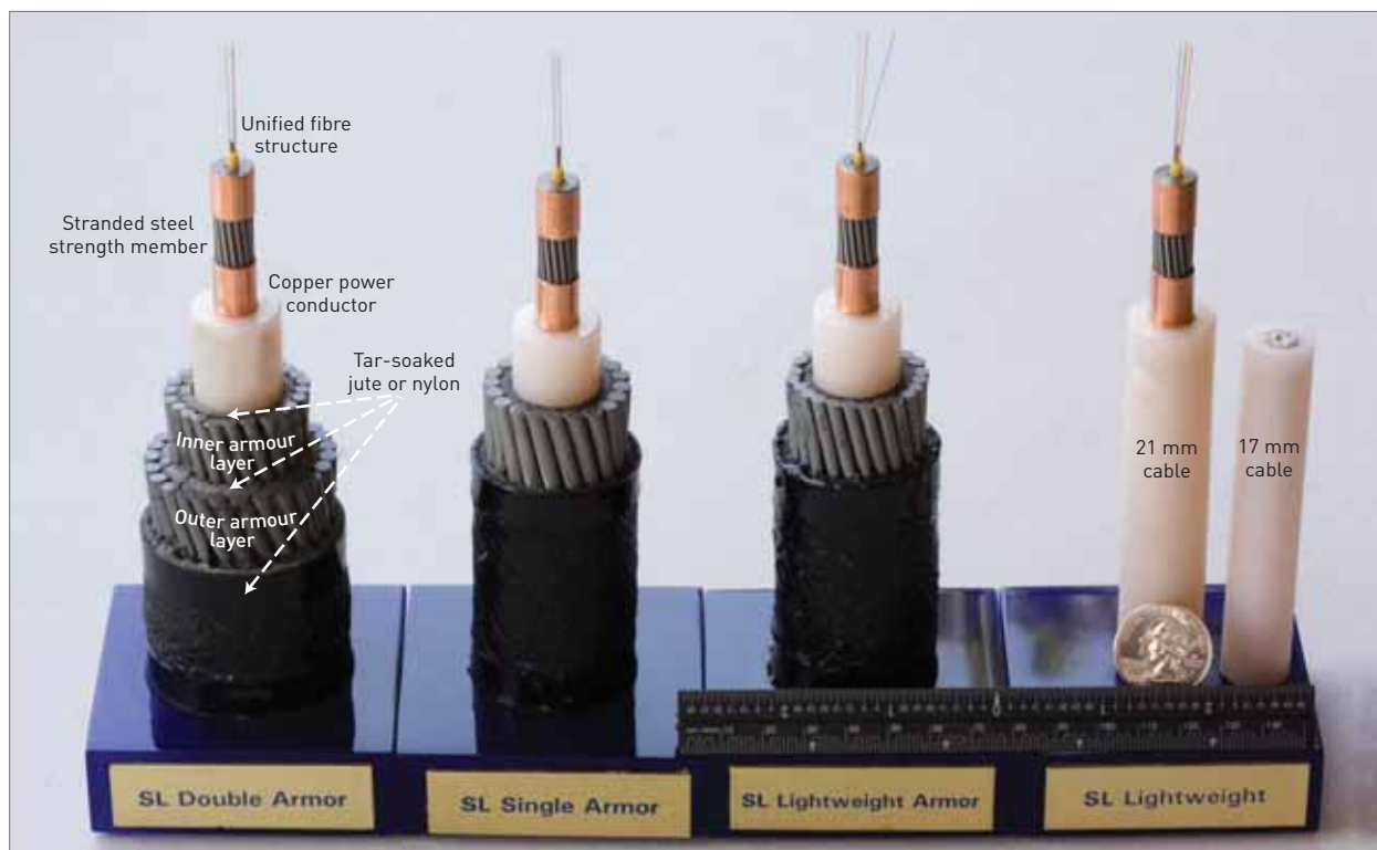
Figure 2.3: Shallow- to deep-water (left to right) fibre-optic cables, with a core supporting pairs of hair-like optical fibres surrounded by a layer of wire to provide strength, a copper conductor to power the repeaters or amplifiers that process the light signal, and a case of polyethylene dielectric. Wire armour is added for protection. Source: Lonnie Hagadorn.
