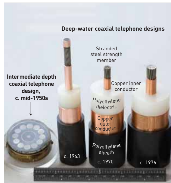
Figure 2.2: Cables of the coaxial telephonic era, with a core of steel wires for strength, an inner copper sheath, which also acted as the conductor, encased in polyethylene dielectric, and an outer conductor. The assembly was coated with black polyethylene which, in shallow water, was armoured for protection. Source: Lonnie Hagadorn.
