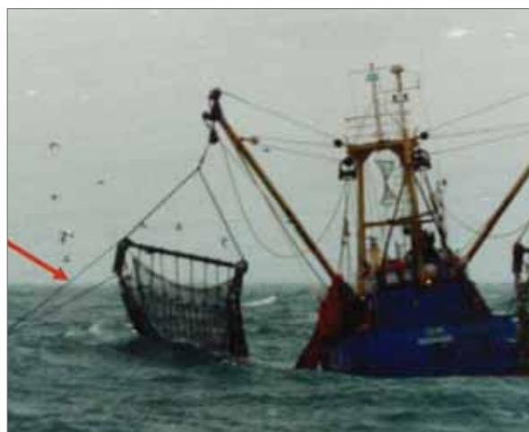
Figure 7.6: Beam trawler with gear snagged on cable (arrow). Snags cause trouble for fishermen, cable companies and users of communications services. Source: Tyco Telecommunications (US) Inc.
