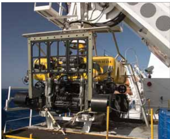
Figure 3.5: TRITON ST-214 remotely operated vehicle (ROV), which is designed to assist burial of cables in areas inaccessible to a sea plough. It also performs cable inspections and recovery operations. Source: Lonnie Hagadorn.
