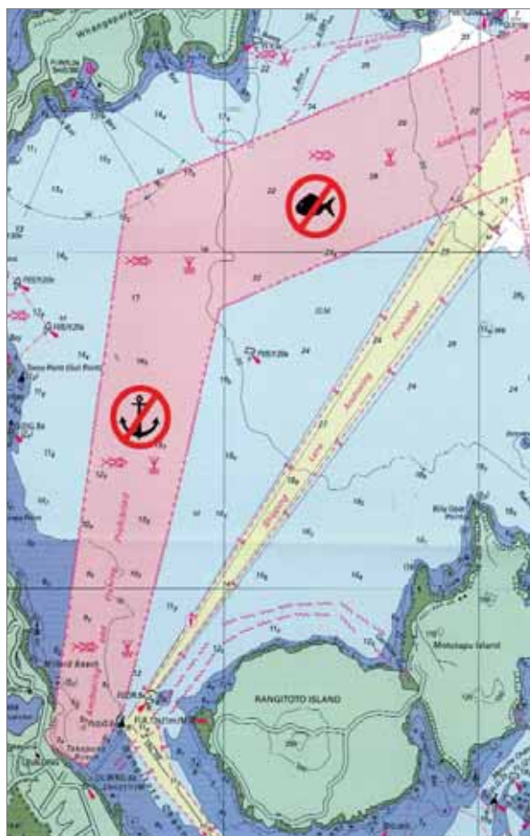
Figure 5.7: Cable protection zone for the New Zealand terminal of the Southern Cross and other international submarine cables. Such protection zones have the potential to act as de facto marine reserves. Source: Telecom New Zealand.
