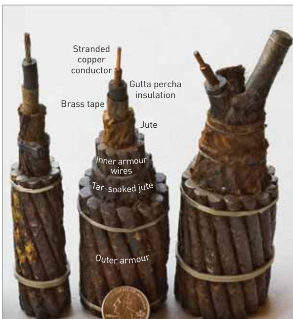
Figure 2.1: Submarine telegraph cables from the early 1900s, with the inner copper conductor for transmitting messages, an insulating layer of the tree resin, gutta percha, and one or more outer layers of iron wire for strengthening and protecting the whole assembly. Source: Lonnie Hagadorn.
