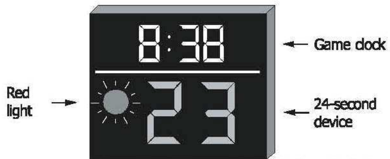
Twenty-four (24) second clock display unit, duplicate game clock, and red light for Levels 1 and 2 (example of the layout)
