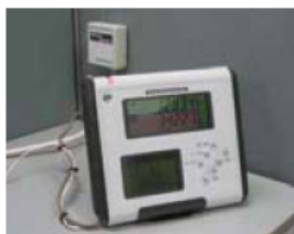
Energy Conservation Navigator (Smart Meter)
