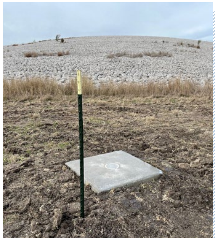
One of the six aerial-survey quality-control monuments at the Falls City, Texas, Disposal Site.
