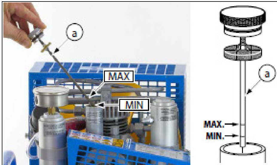
Figure 5. Checking Lubricating Oil Level
