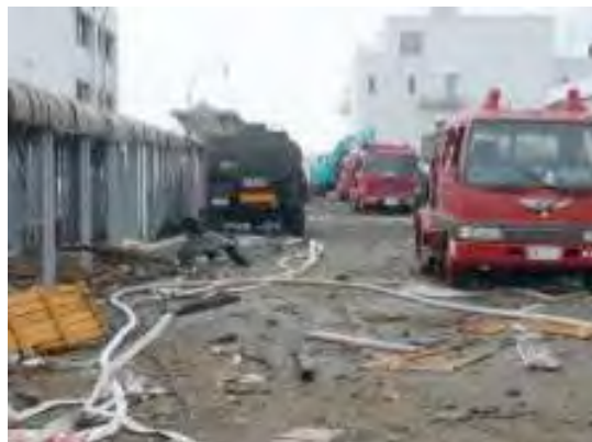
Figure 10: Fire trucks for sea water injection; source: Ref. 44
