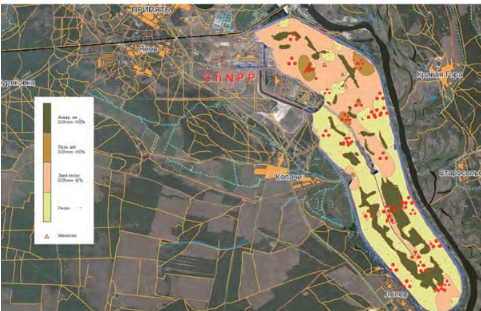
Figure 7-4 Cooling pond at the Chernobyl nuclear power plant with sediments drawn in 59
