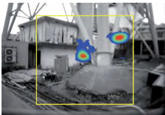
Figure 3-6 Base of stack, units 1 and 2, photographed with a gamma camera 19
