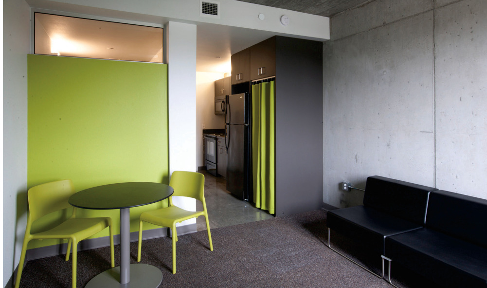
Bud Clark Commons features 130 single-occupant apartments. Each unit is provided with direct ducted outdoor fresh air through rooftop heat recovery systems. Interior windows located high on the wall of the bathrooms allow daylight to penetrate further into the space and provide some natural lighting.
