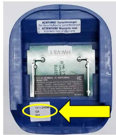
Figure 3 – Determine two-letter Tool Date Code (Circle shows “QS” in this example)
