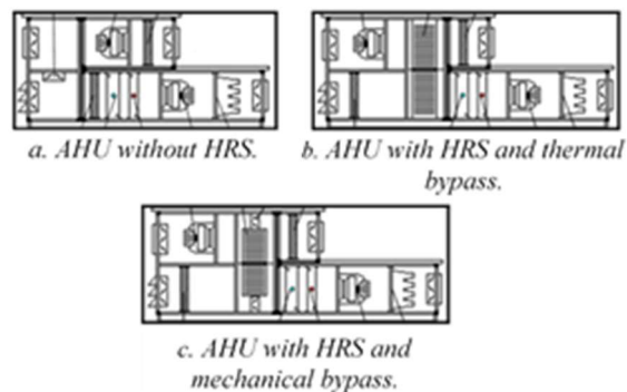
Figure 1. Constructive solution of the AHUs studied.
