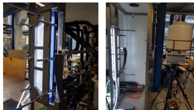
Figure 3: Left) Visualization section. Right) Visualization section and position high speed camera.
