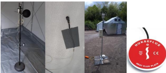
Fig. 3: Left to right; 1. Tripod installed in a small shelter with air temperature and RH sensors and a black globe to measure the MRT at 120 centimeters, and an additional air temperature sensor at 50 centimeters height. 2. Thermistor applied to the center of a roof panel, fixated with iron wire. 3. On-site weather station, 200 centimeter height. Viewing direction to the south. 4. Heat flux plate
