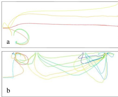
Figure 16. Flow patterns (a) AP-H / AP-D, (b) Mechanical Ventilation
