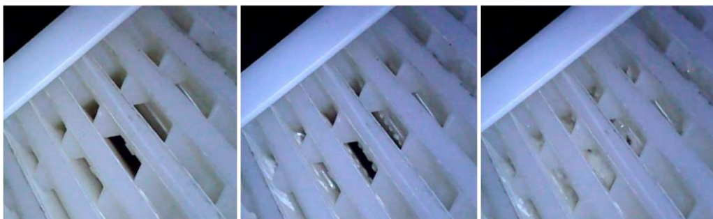
Figure 3. The process of frost formation inside the measured heat exchanger
