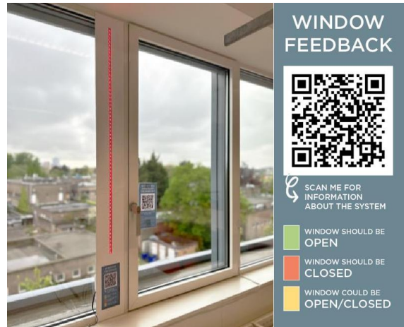
Figure 3. Designed and implemented window feedback system with corresponding legend and QR code
