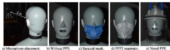
Figure 3 – Experimental setup to assess the impact of PPEs on speech levels. Source: [20].
