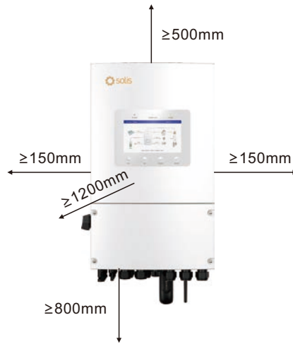
Figure 3.5 Inverter Mounting Clearances
